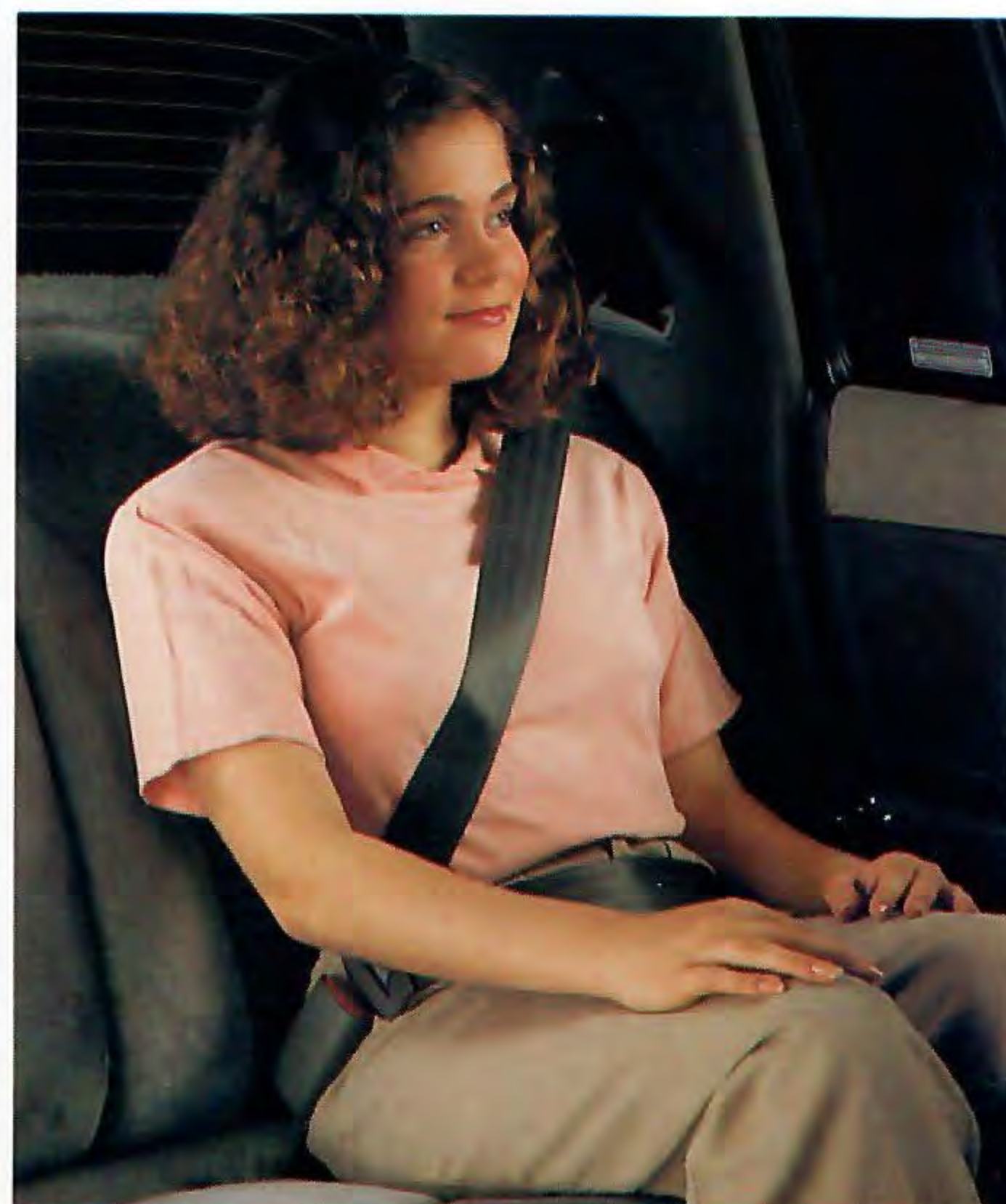
Unibelt three-point shoulder/lap restraints are provided for front and rear outboard passengers.
