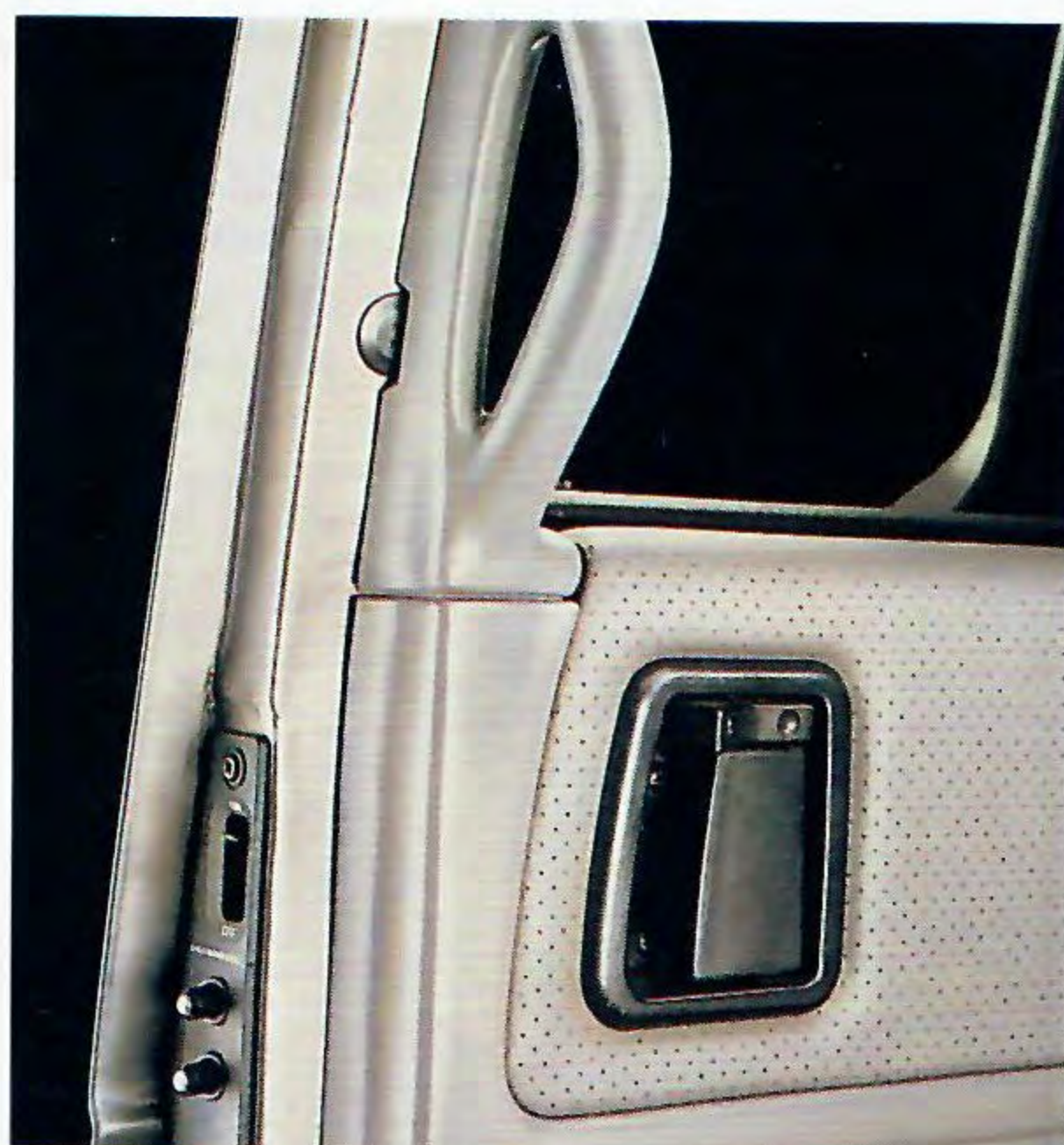
Caravan's sliding side door features a new child guard lock.
